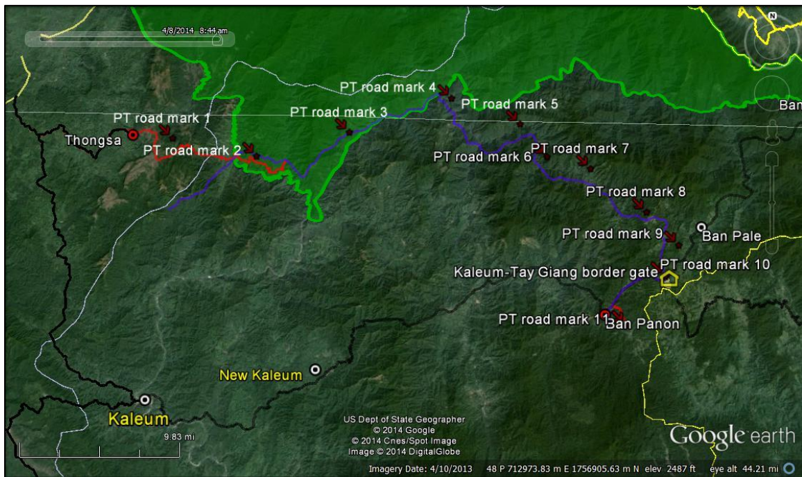
Figure 25. Location of geo-referenced points (“PT road marks”) comparing to road route from the first scheme (blue line). Red line shows already built road.
