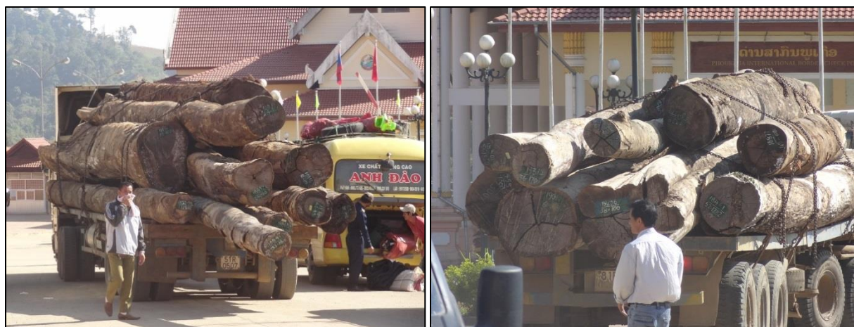
Figure 8. Trucks with round wood in border check point Phou Kua-Bo Y (06 December 2013). Average diameter and length written on log butts allows for calculation of the volume of timber transported by truck: 20.8 m 3 (left) и 24.2 m 3 (right).
